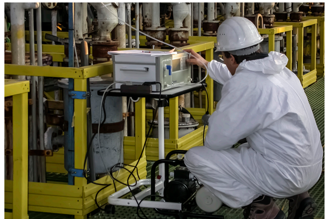
MC-3000 in operation: Calibration of a mercury monitoring system
