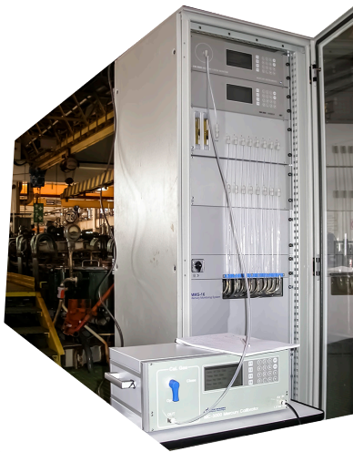
MC-3000 in operation: Calibration of a mercury monitoring system
