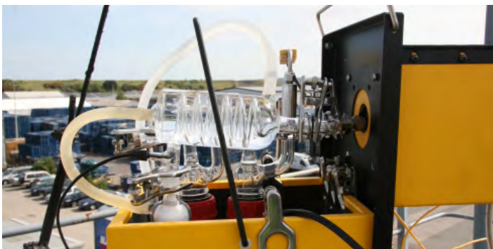
Isokinetic sampling train used to extract particulate samples in order to calibrate particulate monitoring systems
