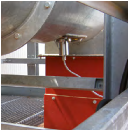
MEASUREMENT ON A SCREW FEEDER
