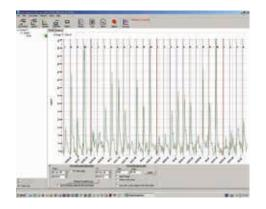
Predict module, sequential pulse cleaning analysis of a bag house chamber with 10 rows. High peaks indicating Bag Row degradation. Ease of access to emissions data from sources plant-wide is vitally important. Dust Tools software is a powerful and customizable software suite for down-loading, displaying, analysing and reporting data from both ENVEA control units and sensors to PCs.
