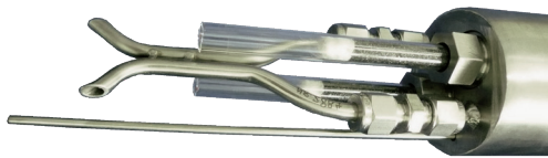
Built-in pitot tube and a thermocouple to sample under volume proportional conditions
