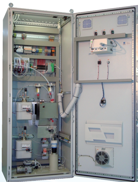
Control cabinet with sample gas conditioning to collect condensate (for moisture calculation) and accurate measurement of volume and flow. IP40 enclosure (54) protects all components - chiller, gas meter, ... - against harsh environmental conditions.
